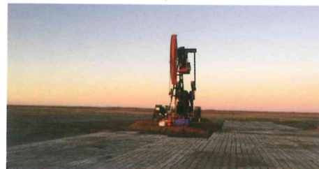
Minimal disturbance drilling sometimes includes the use of matting when on prairie. Photo credit: Sheila Taillon
